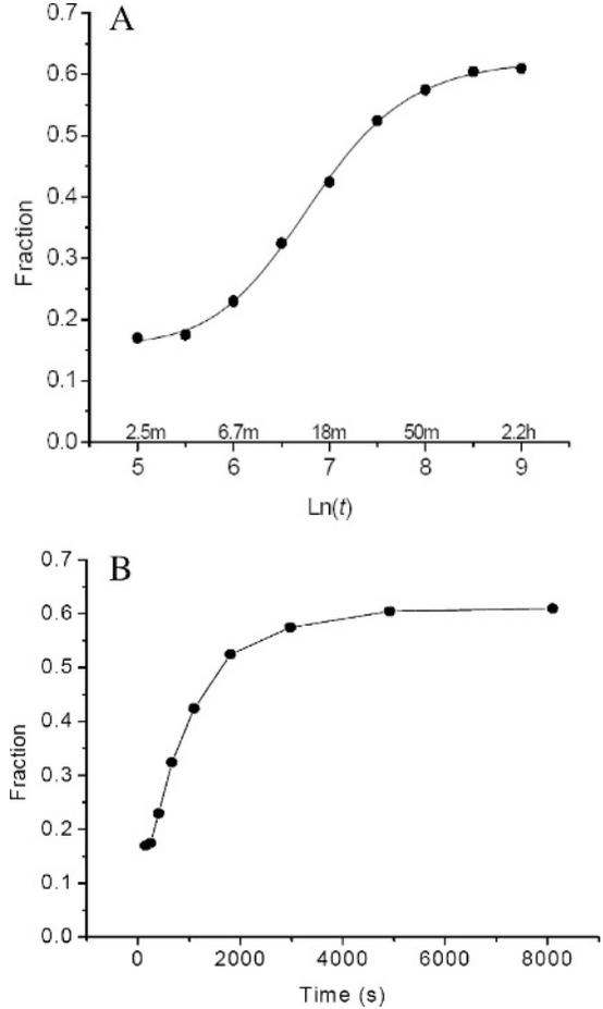
Fig. 3. A time to completion curve in log time (A) and linear time (B) for the real-time solvers for a typical problem.
